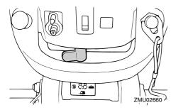
Disconnect the fuel line if you are using an external fuel tank.
